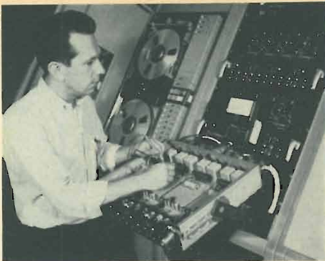
Swing-out chassis on the PAMS console makes servicing easier.
