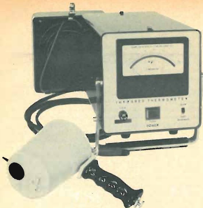
Fig. 4. The infrared thermometer consists of a hand-held or tripod-mounted sensing head (left) containing a thermistor bolometer detector, optical lenses and filters, controlled-temperature chamber, and mechanical chopper. The temperature of the ocean surface can be read directly on the meter located in the case of the instrument. (Barnes Engineering Co.)
